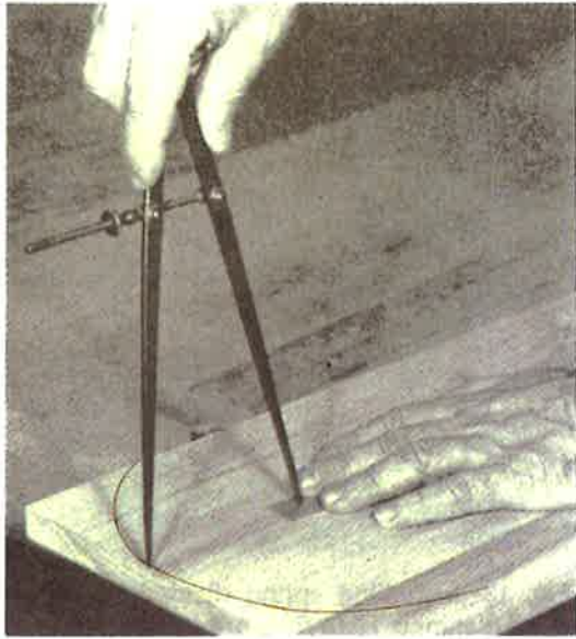
Fig. 13-4. Scribing an arc with dividers. Note the piece of cardboard under the stationary leg to protect the wood grain.
