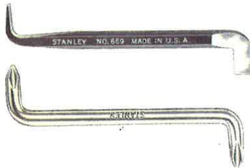
Fig. 19-11. Two types of offset screwdrivers to fit slotted and Phillips-head screws.
