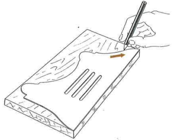
Fig. 14-8. Tracing a pattern on wood around a template.
