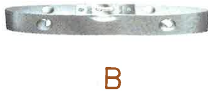
Fig. 7-13. Levels: (A) 24-inch aluminum, (B) 9-inch torpedo.
