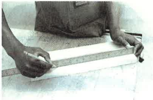
Fig. 7-20. Laying out a measurement with the rule on edge.
