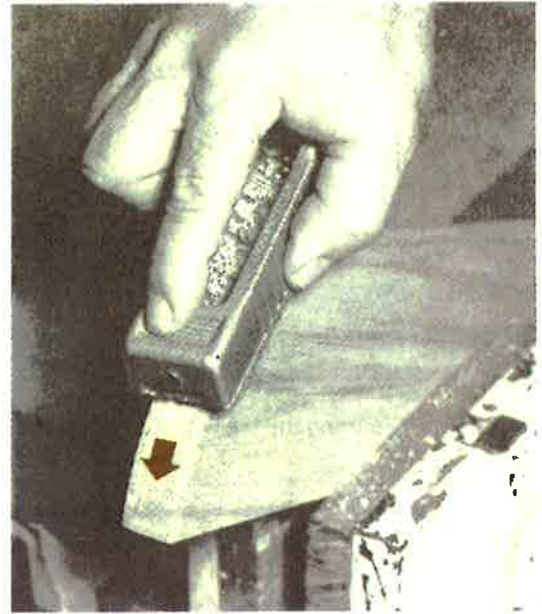
Fig. 14-19. Dressing an edge with a block-plane forming tool.
