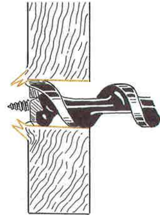
Fig. 18-26. Incorrect boring of a hole.
