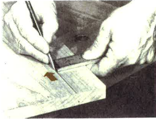
Fig. 7-24. Rule and pencil used as a marking gage.
