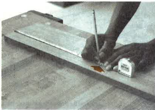
Fig. 7-21. Laying out a measurement with a flexible rule.
