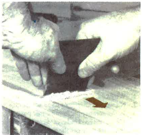
Fig. 17-3. Pulling a scraper blade.
