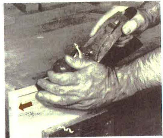
Fig. 11-3. Planing a chamfer.
